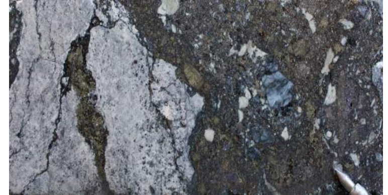
BAR013: 82.90m of 4.18g/t Au & 26.9g/t Ag High-energy matrix-supported polymict breccia within a silica-sericite altered brecciated schist. Milled chaotic clasts. Sulphide content approximately 20%.
