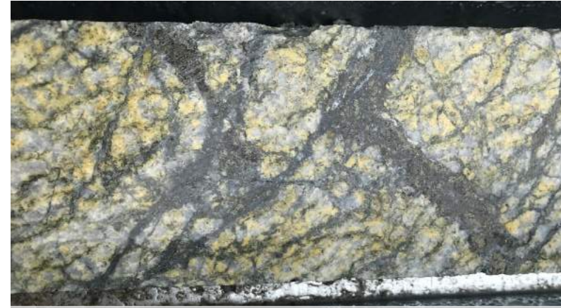
Sulphide-stringers and fracture-fill mineralization (BAR002)
