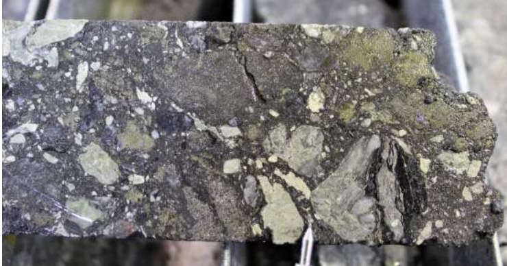
BAR008: 53.30m of 7.19g/t Au & 71.6g/t Ag Matrix-supported sulphide-rich polymict breccia with massive sulphide clasts (galena-sphalerite-pyrite-arsenopyrite). Approximately 15% sulphide content.
