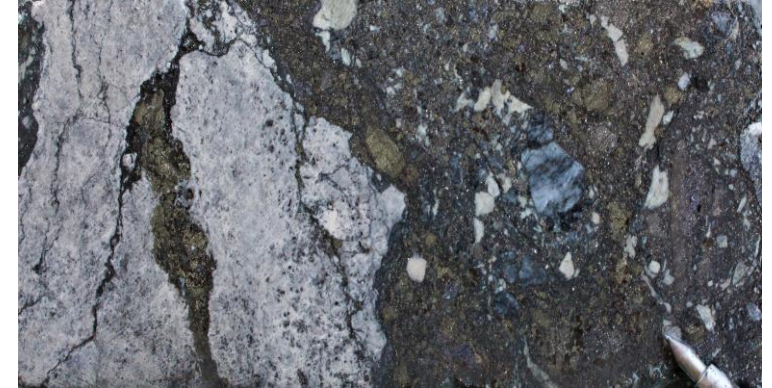
BAR013, 82.90m, 4.18 g/t Au, 26.9 g/t Ag. High-energy matrix-supported polymict breccia within a silica-sericite altered brecciated schist. Milled chaotic clasts. Sulphide content approximately 20%.
