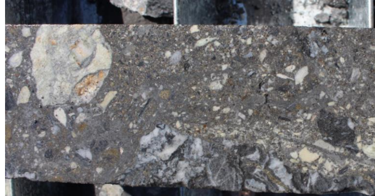
BAR010, 52.60m, 24.70 g/t Au, 1750 g/t Ag. Matrix-supported chaotic polymetallic breccia. Rounded massive sulphide clasts of pyrite-sphalerite-galena range from 0.5cm up to 10cm across sample interval. Pyrite-arsenopyrite rich fine grained matrix.
