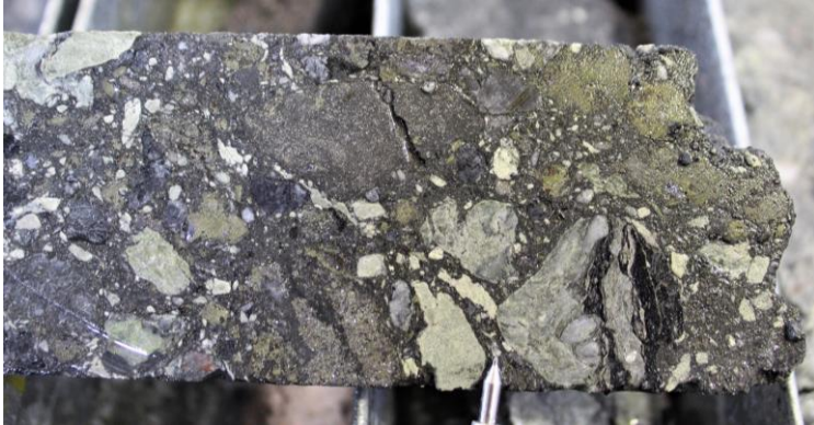
BAR008, 53.30m, 7.19 g/t Au and 71.6 g/t Ag. Matrix-supported sulphide-rich polymict breccia with massive sulphide clasts (galena-sphalerite-pyrite-arsenopyrite). Approximately 15% sulphide content.
